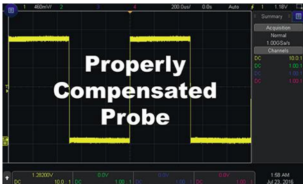
4. Here's what a properly compensated probe should look like.
