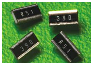
Wide Terminal Current Sense Resistors (WK73S & WU73)
