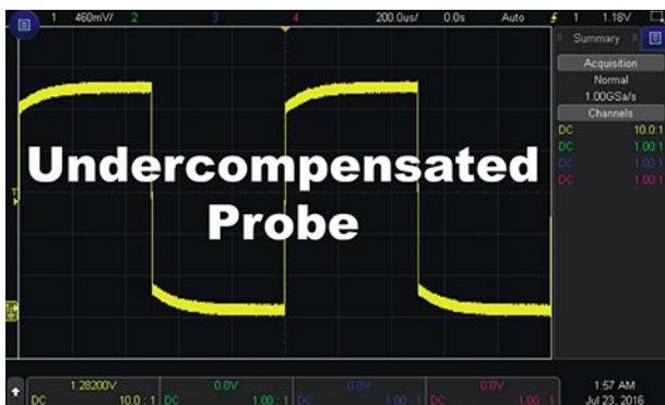
5. This screenshot indicates an undercompensated probe; the signal should be a square wave in this case, too.
