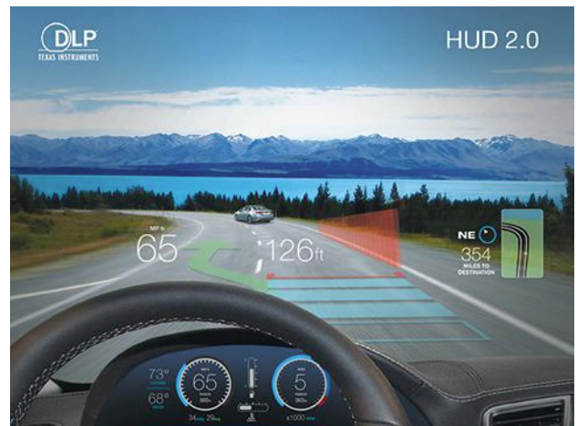
8. Texas Instruments' DLP3000-Q1 digital micromirror device (DMD) and chipset are automotive-qualified and provide a 12-degree field of view.
